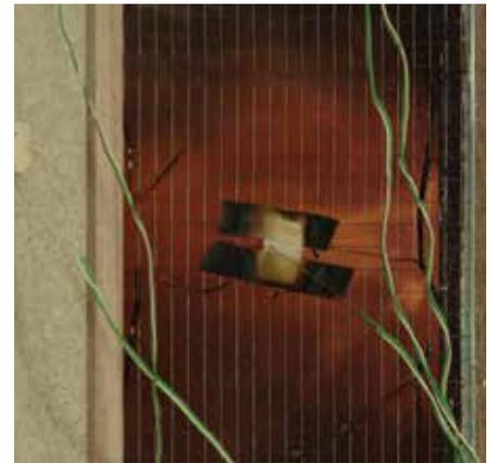
Thermocouples measure a rise in temperature.
