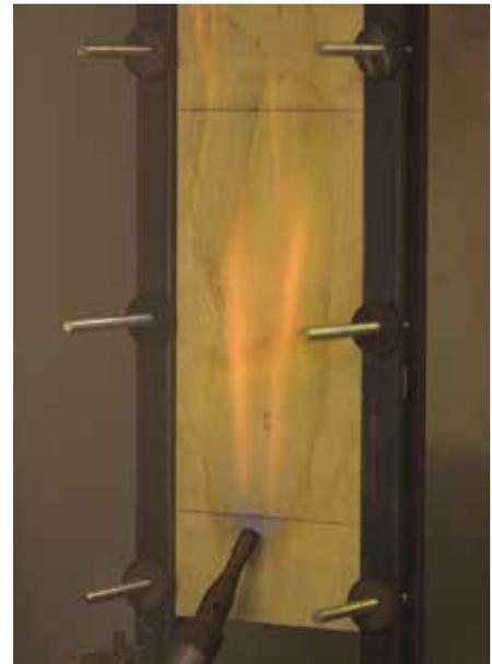
Single flame ignitability test apparatus.
