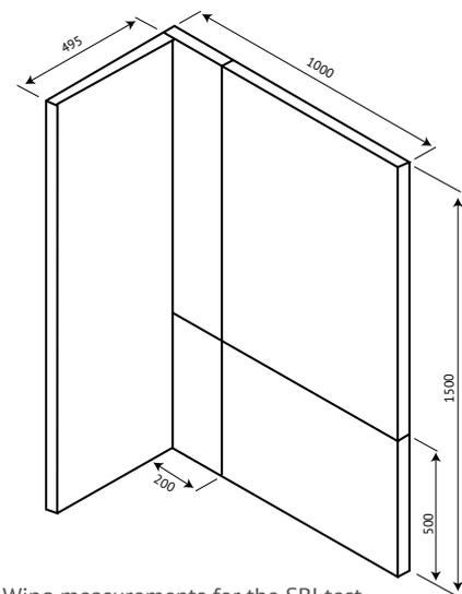
Wing measurements for the SBI test.
