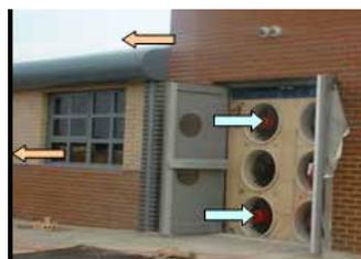
g) Air flow measurements are taken at a range of pressure differentials.
