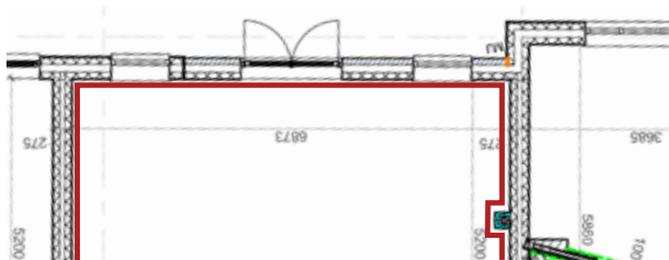
b) The envelope area (EA) is calculated using the drawings (depicted in red) and expressed in m<sup>2</sup>. The EA is based on the internal surface area of the external facades.
