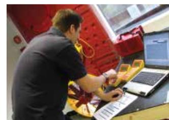
h) Software is used to calculate the air leakage rate.
