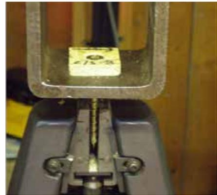
Pull through test to determine the fastener head resistance in materials.
